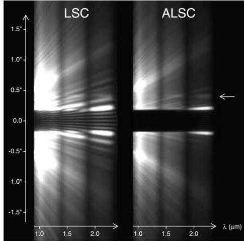
Figure 9: (Vigan et al.) Simulated data with the LSC (left) and ALSC (right) designs representing a 1-hour total integration time on a G0 star at 10 pc. A fake companion ( $T_{eff} = 1400$  K,  $\log g = 5.0$ ) has been introduced at a separation of  $+0.4''$  from the star (left pointing arrow). Strong diffraction residuals are clearly visible on either side of the coronagraphic mask for the LSC, while the apodizer has almost completely suppressed diffraction for the ALSC.
